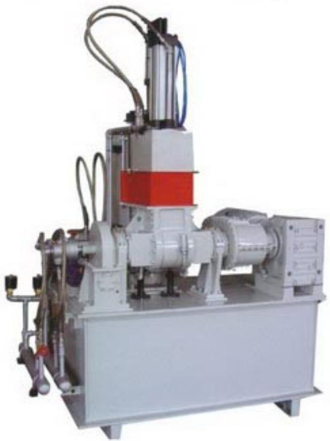
**Non-Pressure Mixing Roll of Open Type 3L**
