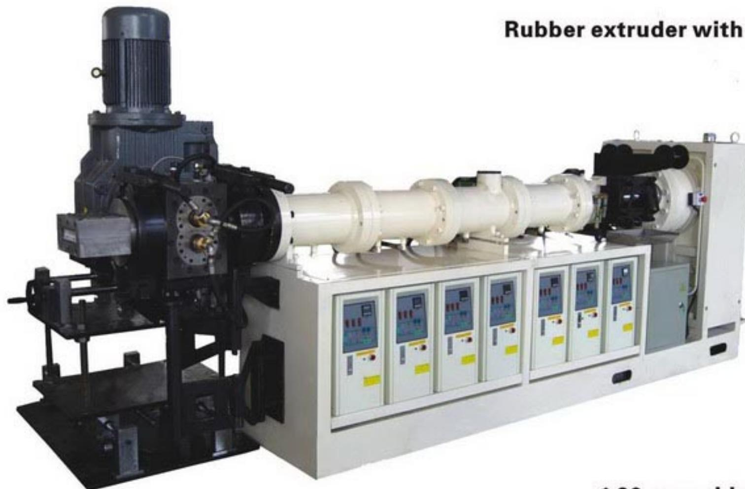
Rubber extruder with gear pump
