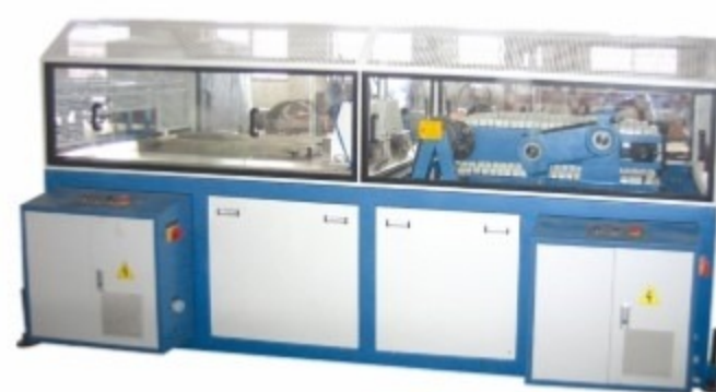
Double Pipe Haul-Off and Cutting Unit
